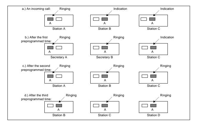
A call rings on Station A. If Station A does not answer within a preprogrammed time, the call also rings on Station B. If the call is not answered within the second preprogrammed time, the call also rings on Station C. If the call is not answered within the third preprogrammed time, the call also rings on Station D.
