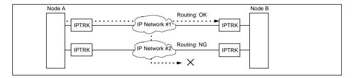
7. When multiple IPTRK cards are used for node-to-node connection and all the lines on an IPTRK are busy, alternate routing is available (see the following figure). However, if a router or FCH-FGH card cannot be used, all the related IPTRK routes are also made unavailable.
