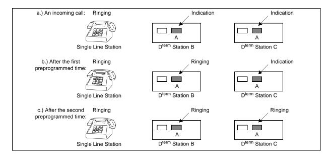
A call rings on Single Line Station A. If Station A does not answer within a preprogrammed time, the call also rings on D<sup>term</sup> Station B. If the call is not answered within the second preprogrammed time, the call also rings on D<sup>term</sup> Station C.
